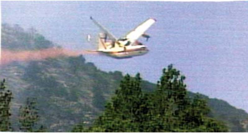
Fig. 14-1. A C-130 forest-fighting plane in the process of losing its wings.
