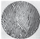
Coarse pearlite formed at about 720°C (Mag ~2,500×)
